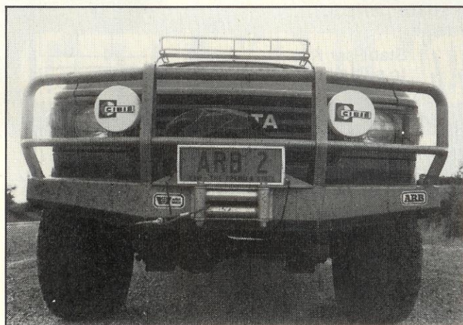
Large bull bars can carry a fuel penalty unwarranted in all but "serious" off-road use.
