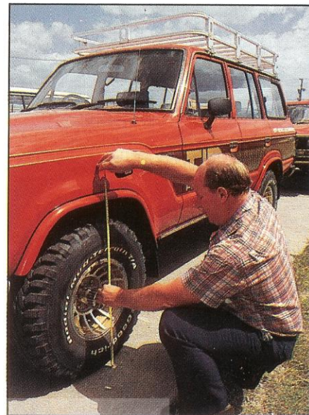
Measuring up the difference in ride height between standard (left) and modified (right) LandCruisers.
