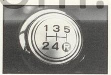
At first we thought it was a modified Dyna box, but further investigation showed that it was a completely new unit. The first four ratios are in fact the same as the previous model; the indirect fifth being the new addition. Gear ratios are: 1st 4.843; 2nd 2.619; 3rd 1.516; 4th 1.00; 5th 0.845; Rev 4.843; Final Drive 4.111.
