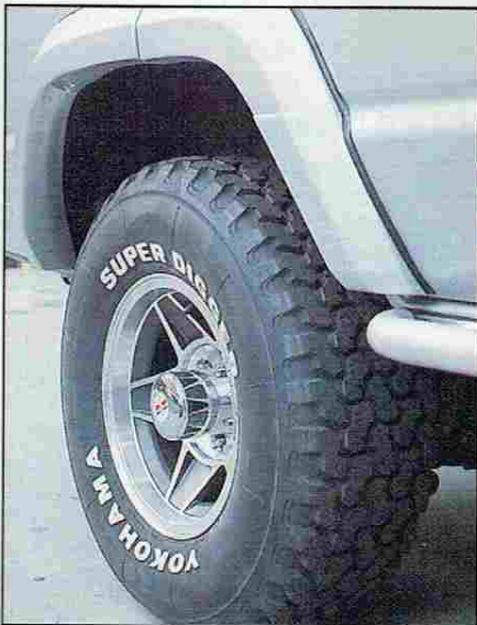
Fitting wider wheels and tyres often calls for flares. These Sahara replicas in fibreglass were obtained from Opposite Lock, fitted by ARB.
