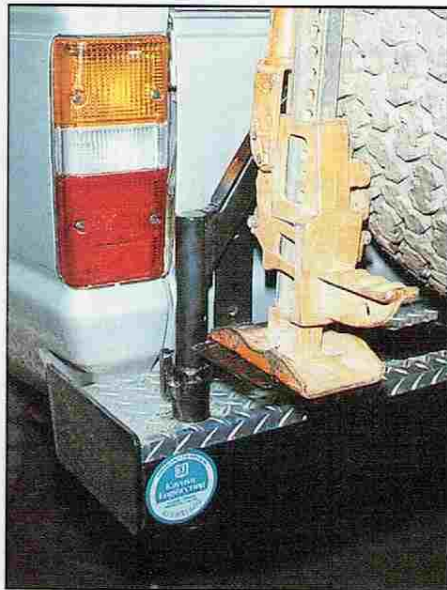
Roofrack was chosen for full length mounting. If it comes off, the roof comes with it! Step bumper and wheel carrier also features Kaymar's Jackall mount.
