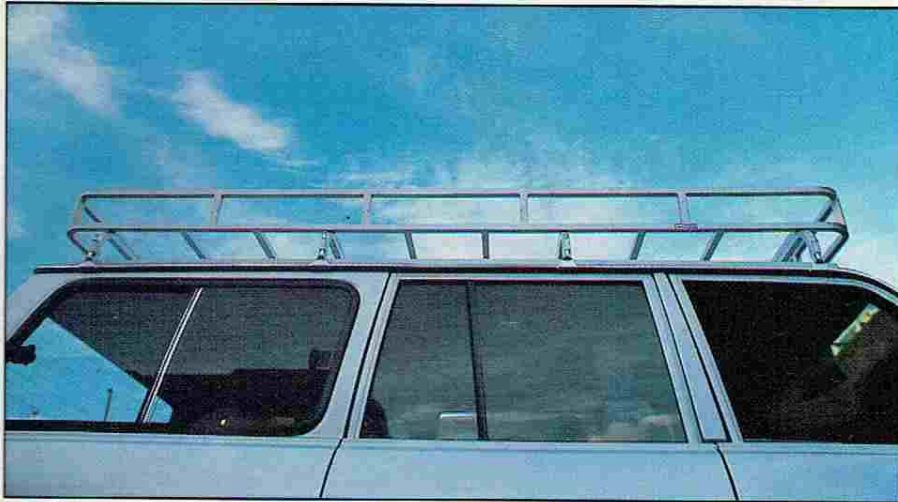
Roofrack was chosen for full length mounting. If it comes off, the roof comes with it! Step bumper and wheel carrier also features Kaymar's Jackall mount.
